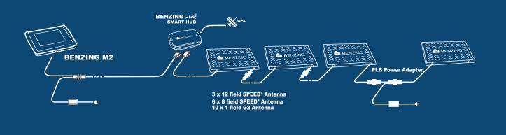
The system can be extended to a maximum of 8 PLB Speed<sup>2</sup> or G2 Antennas at any time using the PLB Power Adapter.
