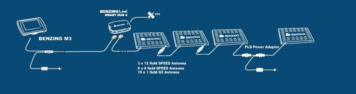
The system can be extended to a maximum of 64 PLB SPEED or G2 Antennas at any time using the PLB Power Adapter.
